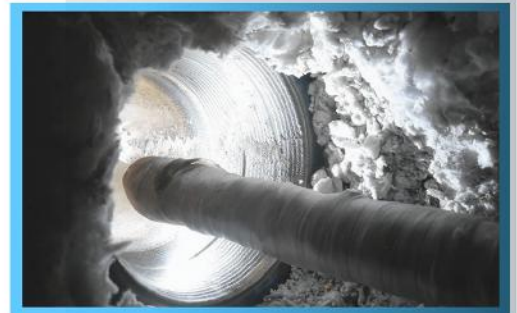
Pipe and Valve ID with corrosion resistance overlay
